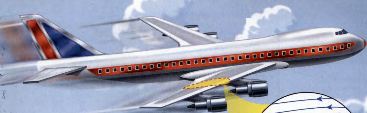
FIGURE 17 Airplane Wing An airplane wing is designed to produce an upward force for a plane in flight. Interpreting Diagrams Why is the pressure lower above the wing?
