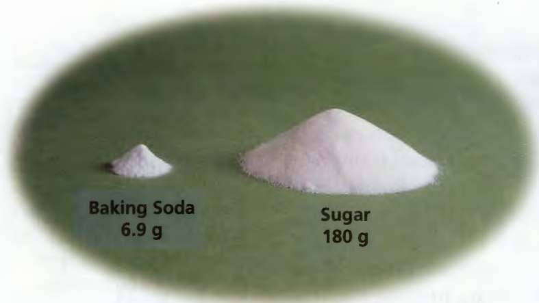
FIGURE 7 Each compound listed in the table dissolves in water, but in different amounts.
