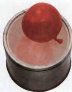
B The balloon is lowered into liquid nitrogen at -196^{\circ}\text{C} .
